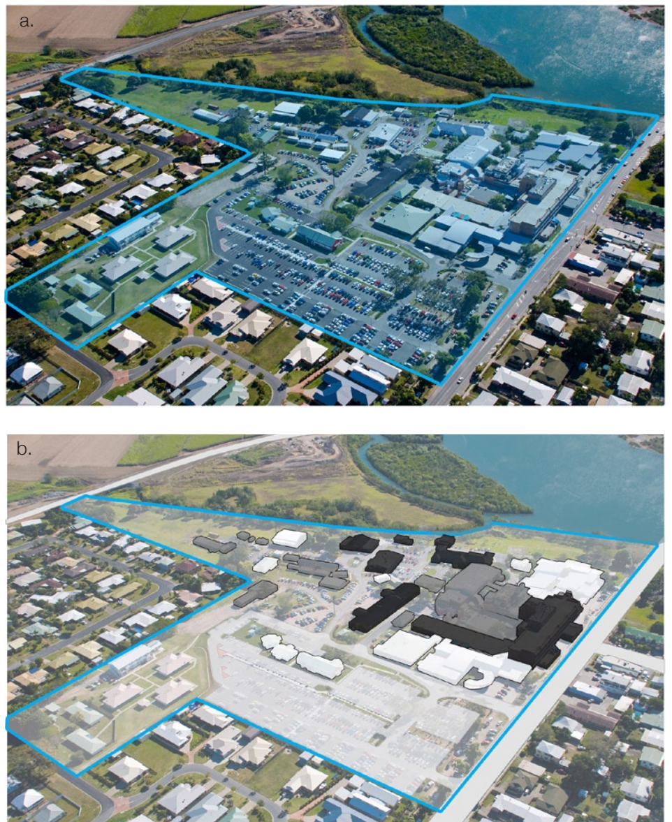
Figure 5. a. The existing Mackay Base Hospital site. b. The revised site plan using the RRDAT Tool. Those buildings shaded in white denote retention potential; those in grey denote refurbishment potential; and those in black denote demolition.
